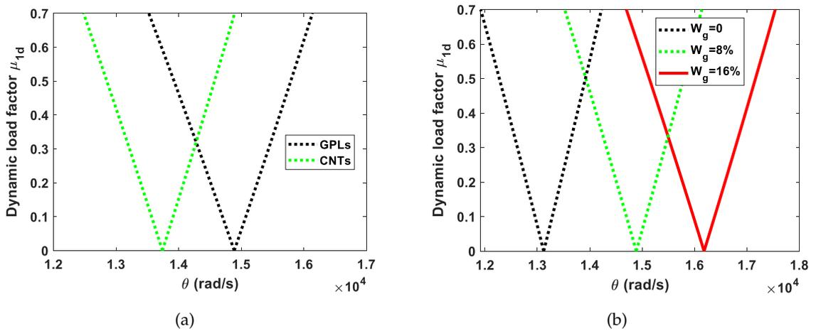
Fig. 4. Effect of core-reinforcement material models (a) and the mass fraction of graphene (b) on the DIR of the DSEM shell
