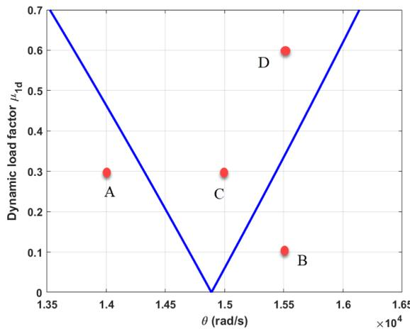
Fig. 2. Dynamic instability region (DIR) of the DSEM shell with a nanocomposite core
