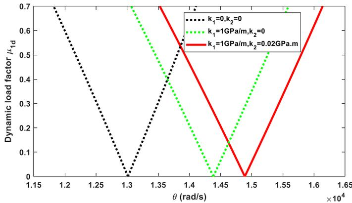
Fig. 6. Impact of elastic foundation parameters on the DIR of the DSEM shell
