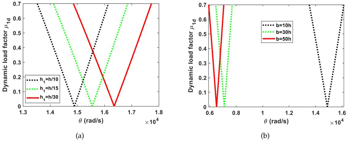
Fig. 5. Effect of electromagnetic layer thickness ratios and width-to-thickness ratio on the DIR of the DSEM shell
