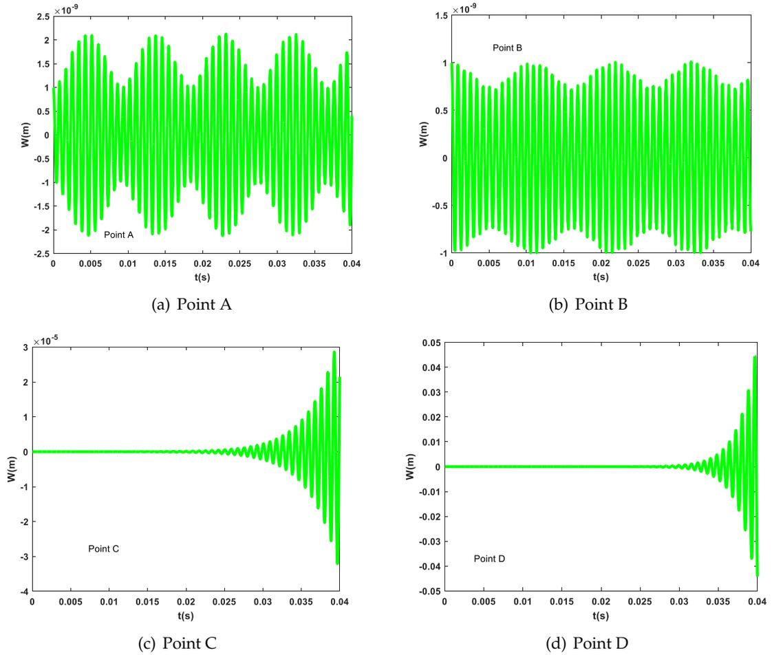
Fig. 3. Time-deflection responses of the DSEM shell under different load cases
