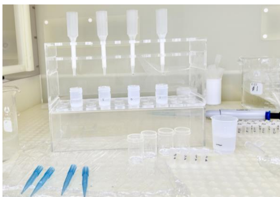
Figure 4. Eichrom Ln-spec resin in 10 ml Nalgene columns for separation of Nd, Sm, and Hf metals.
