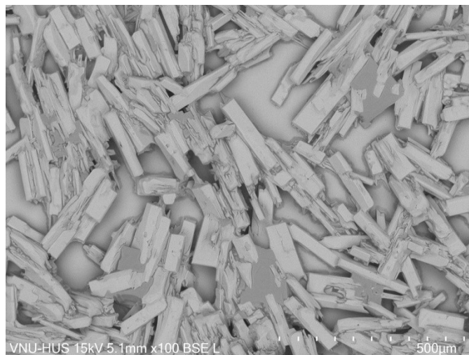
Figure 1. SEM micrograph of 0D \text{FA}_4\text{PbBr}_6 crystals.
