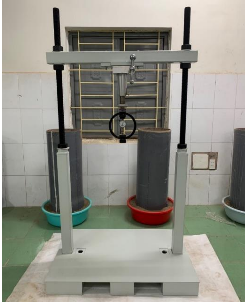
Figure 6. Loading frame system for single stone column
