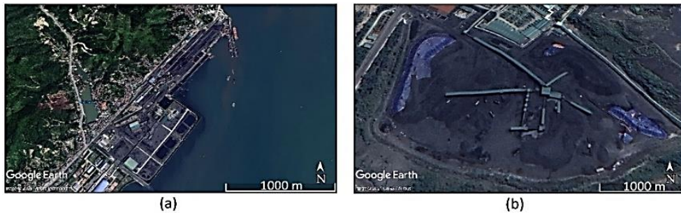
Figure 8. Features on the high-resolution image of the Google Earth dataset: (a) Vessels at coal ports (b) Conveyor belts in coal mines
