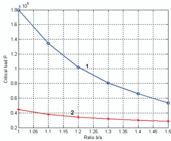
Fig. 3. Effect of plate dimension ratio on buckling load
