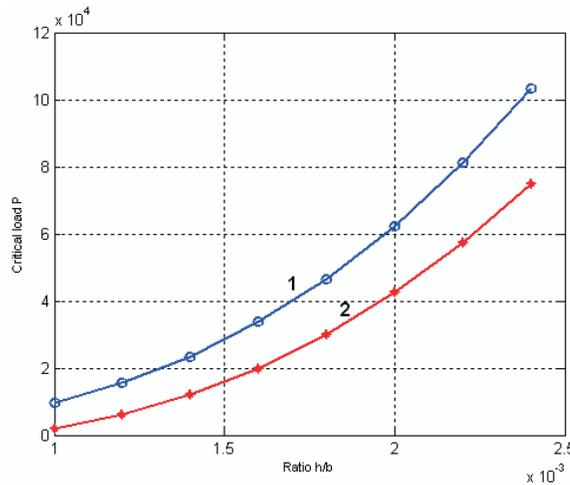
Fig. 2. Effect of plate thickness on buckling load
