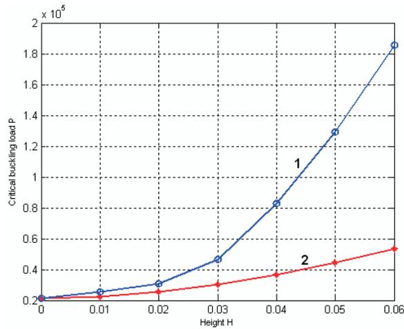
Fig. 4. Effect of the height on buckling load
