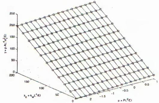
Fig. 4. Influence of axial force and foundation stiffness on frequency parameter of fully supported CF beam
