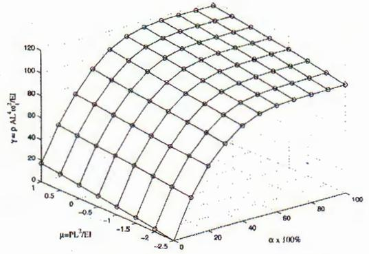
Fig. 8. Frequency parameter of partially supported CF beams at various values of axial force parameter and supporting percentages ( $k_0 = 100$ )
