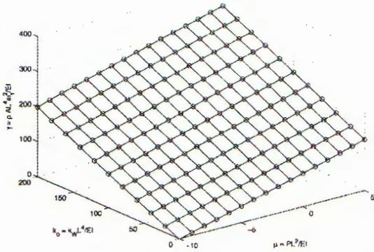
Fig. 3. Influence of axial force and foundation stiffness on frequency parameter of fully supported SS beam
