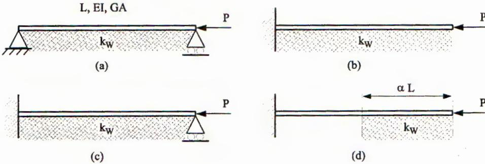
Fig. 2. Beams with with shear deformation for numerical investigation
