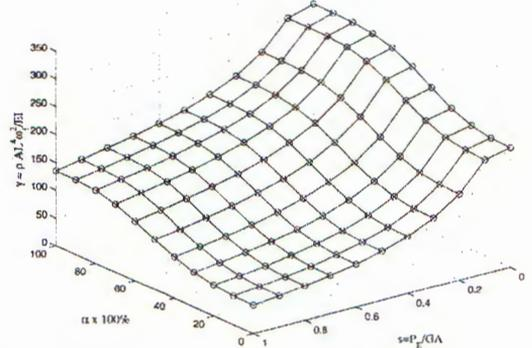
Fig. 12. Frequency parameter of partially supported CS beams at different supporting percentages and various values of slenderness parameter ( $\mu = -2$ ,  $k_0 = 100$ )
