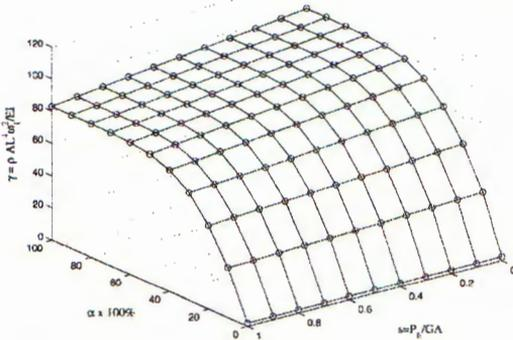
Fig. 11. Frequency parameter of partially supported CF beams at different supporting percentages and various values of slenderness parameter ( $\mu = -2$ ,  $k_0 = 100$ )
