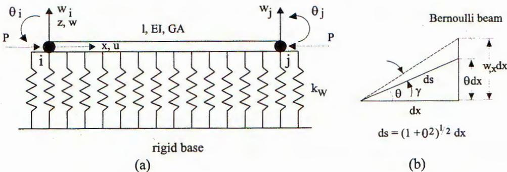
Fig. 1. (a) A two-node beam element, (b) Geometric relation for a differential element of length  $dx$
