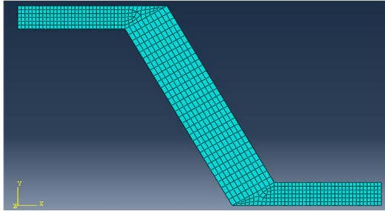
Fig. 3. A meshing on a quarter of the unit cell  $Y$  using a linear plane strain element CPE4R
