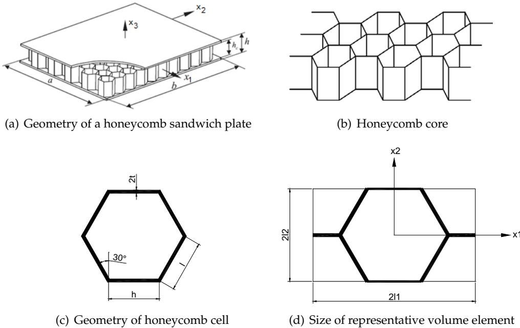
Fig. 1. Geometry of a representative volume element of honeycomb core of sandwich plate
