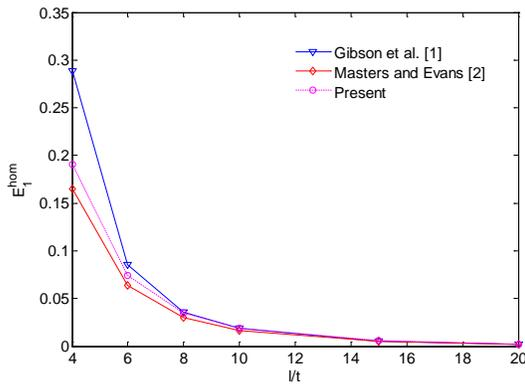
Fig. 4. Variation of homogenized Young's modulus  $E_1^{\text{hom}}$ (GPa) with respect to  $l/t$
