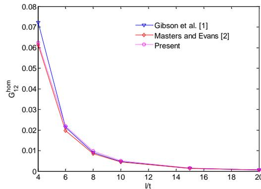
Fig. 6. Variation of homogenized shear modulus  $G_{12}^{\text{hom}}$  (GPa) with respect to  $l/t$
