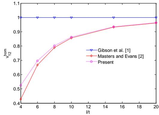
Fig. 5. Variation of homogenized Poisson's ratio  $\nu_{12}^{\text{hom}}$  with respect to  $l/t$
