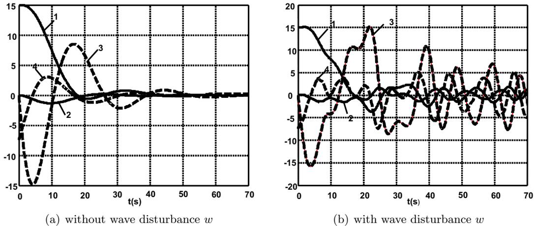
Fig. 4. Closed - loop system characteristics: 1 - yaw angle  $\varphi$  (deg), 2 - yaw rate  $\omega$  (deg/s), 3 - rudder angle  $\delta$ (deg), 4 - control signal  $u$ (deg/s)
