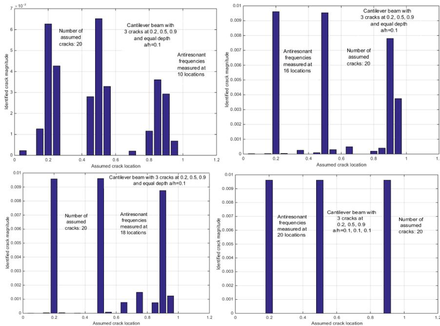
Fig. 3. Results of crack detection by antiresonant frequencies measured at 10, 16, 18, 20 positions on cantilever beam with three cracks at location  $e/L = 0.2$ ;  $0.5$ ;  $0.9$  of equal depth  $a/h = 10\%$ , using model with 20 crack mesh
