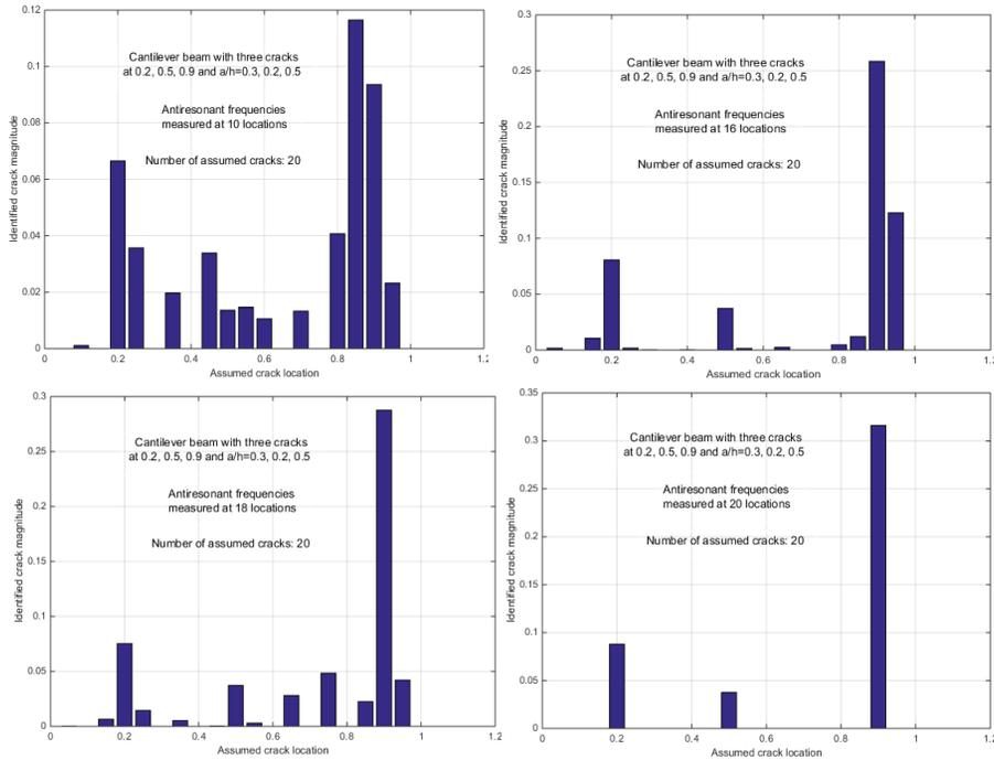
Fig. 4. Results of crack detection by antiresonant frequencies measured at 10, 16, 18, 20 positions on cantilever beam with three cracks of depth  $a/h = 30\%$ ;  $20\%$ ;  $50\%$  at locations  $e/L = 0.2$ ;  $0.5$ ;  $0.9$  using model with 20 crack mesh
