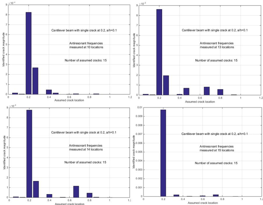
Fig. 1. Results of crack detection by antiresonant frequencies measured at 10, 13, 14, 15 positions on cantilever beam with single crack at location  $e/L = 0.2; a/h = 10\%$ , using model with 15 crack mesh
