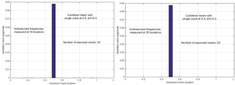
Fig. 2. Results of crack detection by antiresonant frequencies measured at 10, 16, 18, 20 positions on cantilever beam with single crack at location  $e/L = 0.5$ ;  $a/h = 30\%$ , using model with 20 crack mesh
