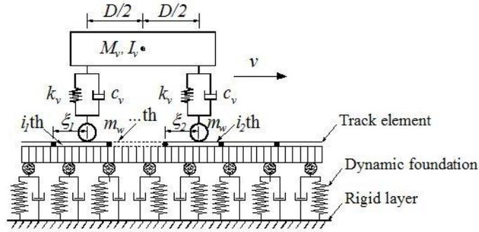
Fig. 3. Model of a railway vehicle-track-foundation interaction element
