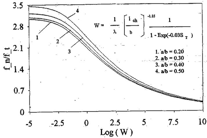
Fig. 3. General size effect curves for beams in bending
