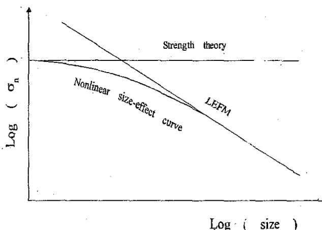
Fig. 1. Assumed size-effect curve on concrete
