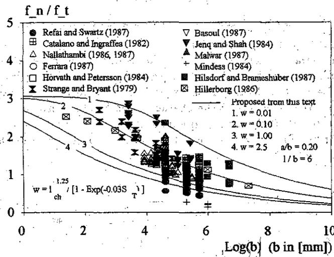
Fig. 4. Checking the size effect law by test and calculation data
