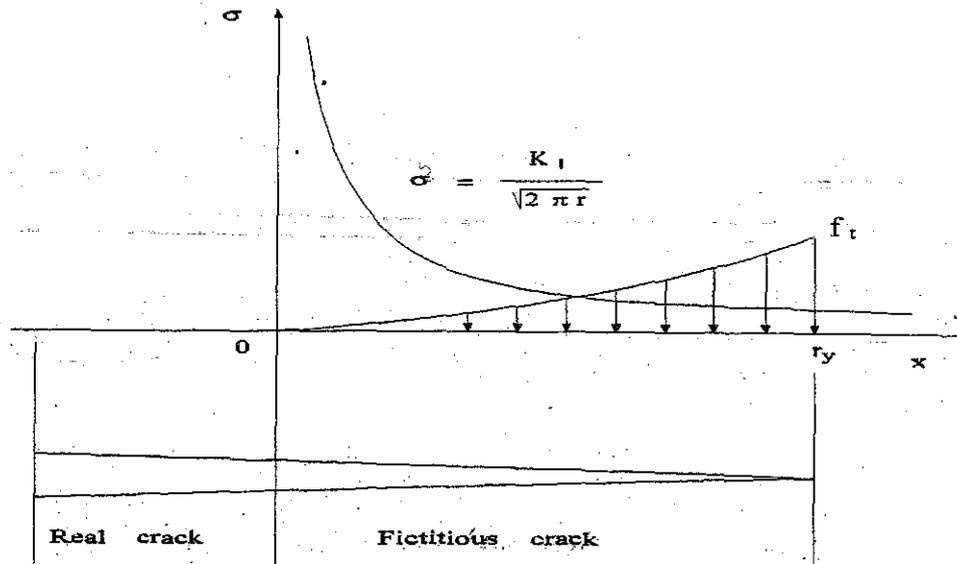
Fig. 2. Stress distribution and the fracture process zone in front of a crack tip
