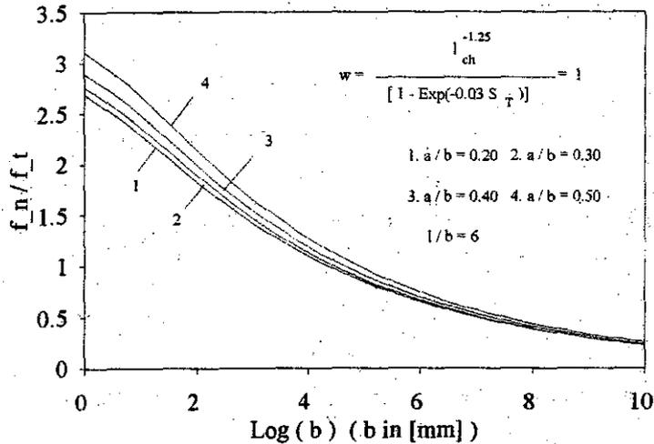
Fig. 5. Influence of the notched depth on the size effect of the nominal strength
