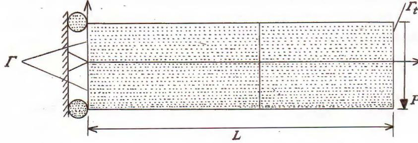
Fig. 1. A cantilever beam 2-D for comparison with the analytic solution from Timoshenko and Goodier
