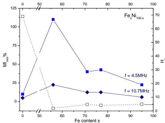
Fig. 5: Influence of Fe content ( $x$ ) on  $MI_{\text{max}}$  (solid curves) and  $H_c$  (dashed curve) of the electrodeposited wires  $\text{Fe}_x\text{Ni}_{100-x}/\text{Cu}$  ( $x = 0 - 95$ )
