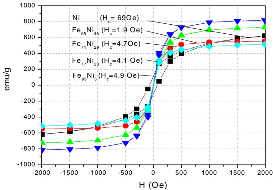
Fig. 3: Hysteresis loop of the electrodeposited wires  $\text{Fe}_x\text{Ni}_{100-x}/\text{Cu}$  ( $x = 0 - 95$ )
