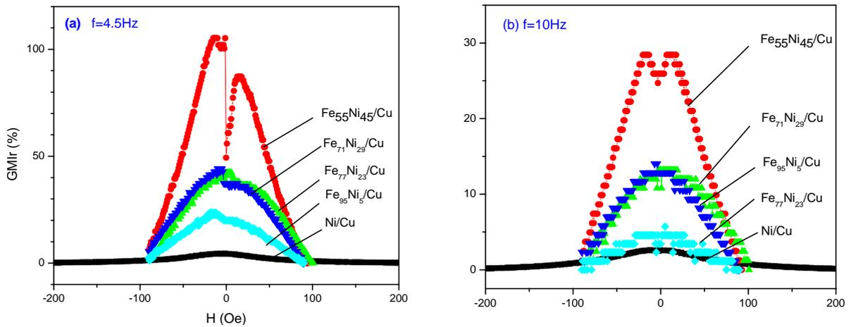
Fig. 4: MI curves of the electrodeposited wires  $\text{Fe}_x\text{Ni}_{100-x}/\text{Cu}$  ( $x = 0 - 95$ )
