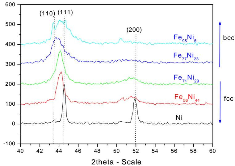
Fig. 2: XRD patterns of electrodeposited  $\text{Fe}_x\text{Ni}_{100-x}$  ( $x = 0 - 95$ ) alloys
