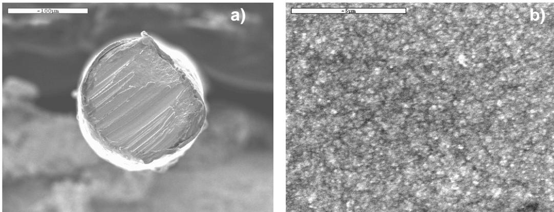
Fig. 1: SEM images of  $\text{Fe}_{55}\text{Ni}_{45}/\text{Cu}$  composite wire
