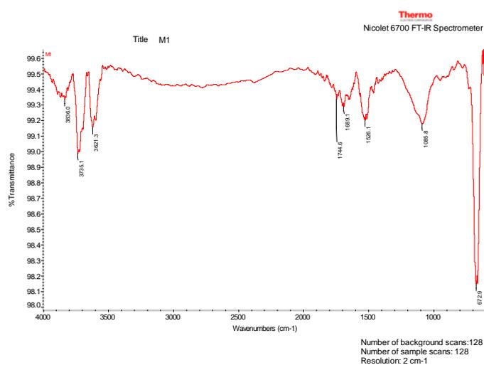
Fig. 2: FTIR spectra (swept range 4000 - 600  $\text{cm}^{-1}$ ) of the bonds DNA- APTS
