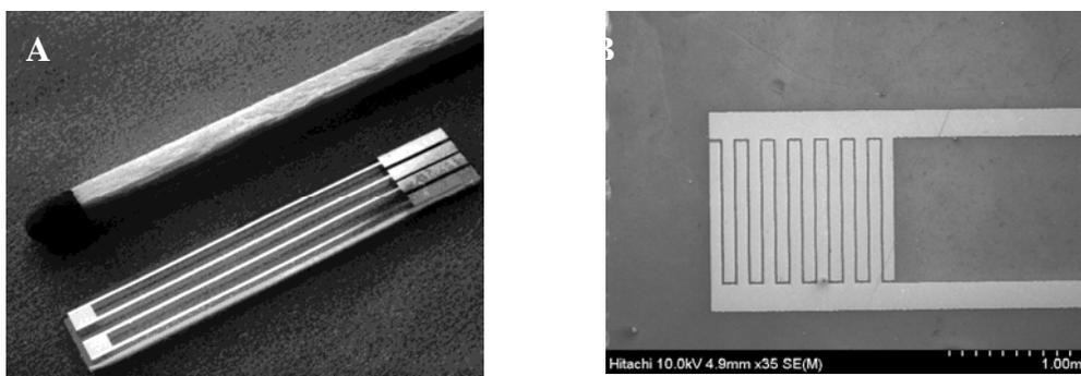
Figure 1: SEM image of an Au micro-electrode
