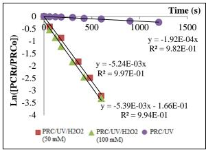
Figure 2: The pseudo first order rate constant of PRC/UV and PRC/UV/H<sub>2</sub>O<sub>2</sub> processes
