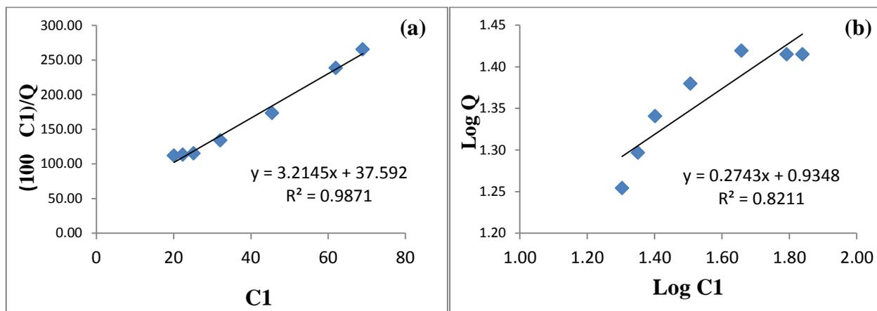
Figure 6: Cd<sup>2+</sup> adsorption isotherm using FA treated by NaOH (pH = 13) solution: Langmuir model (a) and Freundlich model (b)
