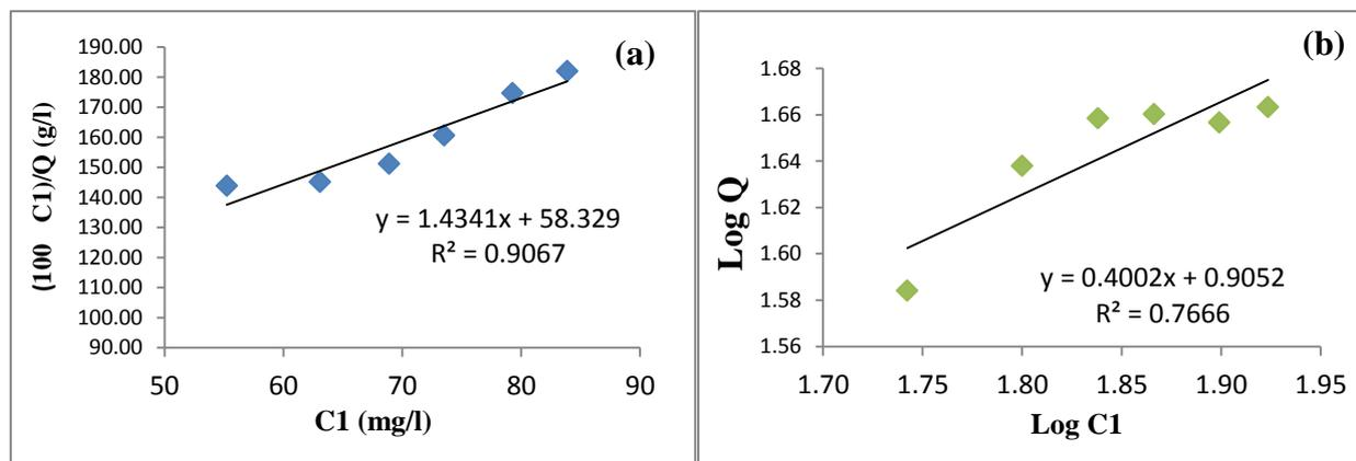
Figure 5: Hg<sup>2+</sup> adsorption isotherm using FA treated by NaOH (pH = 13) solution: Langmuir model (a) and Freundlich model (b)
