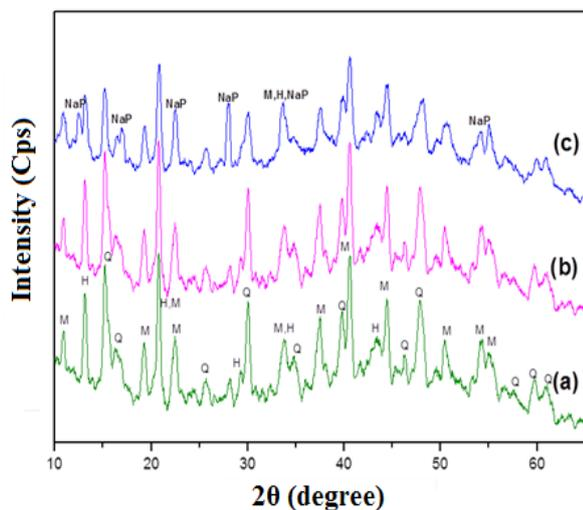
Figure 3: XRD patterns of FA (a), FA treated by H<sub>2</sub>SO<sub>4</sub> solution (b) and NaOH solution (c)
