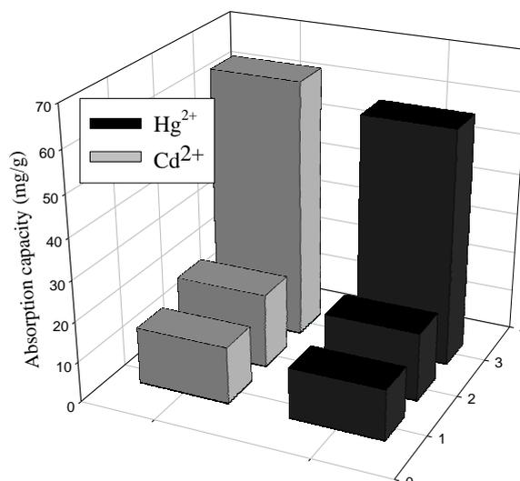
Figure 4: Adsorption capacity of Hg<sup>2+</sup> and Cd<sup>2+</sup> ions by FA and treated FA, 1: FA, 2: H-FA, 3: N-FA
