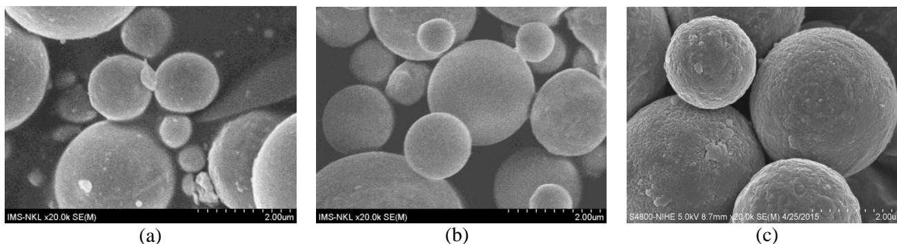
Figure 2: FESEM images of FA (a), FA treated by  $\text{H}_2\text{SO}_4$  solution (b) and NaOH solution (c)
