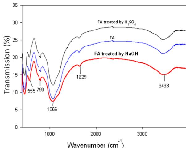
Figure 1: FTIR spectra of FA and FA treated by  $\text{H}_2\text{SO}_4$  - and NaOH solutions
