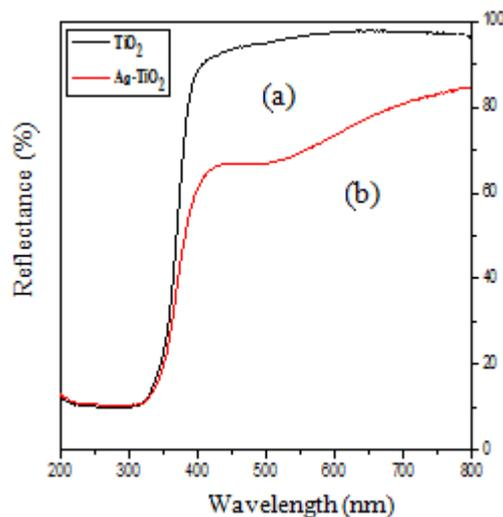
Figure 3: Diffuse reflectance spectra of TiO<sub>2</sub> (a) and Ag-TiO<sub>2</sub> (b)
