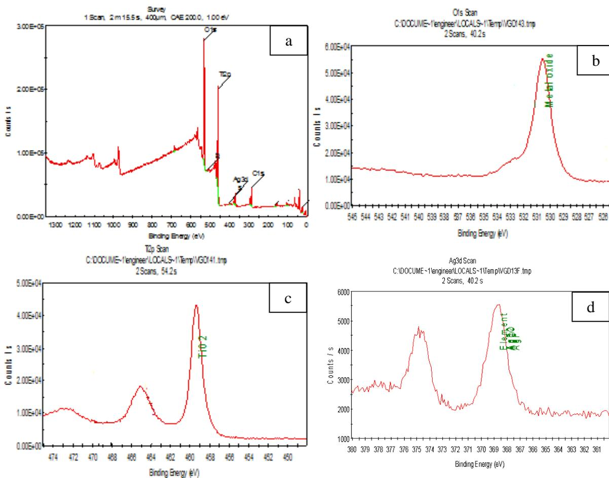
Figure 4: XPS spectra of Ag-TiO<sub>2</sub>
