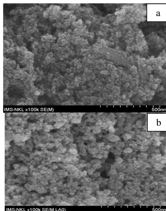
Figure 2: SEM image of TiO<sub>2</sub> (a) and Ag-TiO<sub>2</sub> (b)
