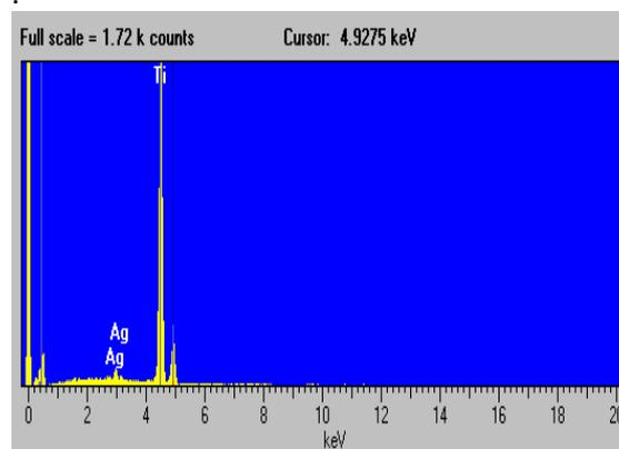
Figure 1: EDS spectrum of Ag-TiO<sub>2</sub>
