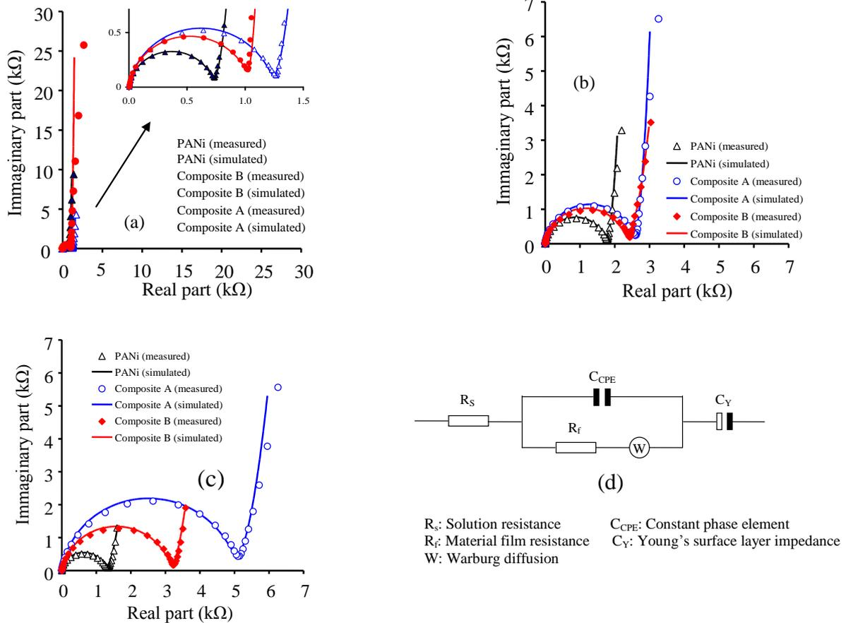
Figure 2: Nyquist diagrams of TiO<sub>2</sub>-PANi composites prepared under different conditions (mass ratio of TiO<sub>2</sub> to aniline: 1/6 (composite A) and 1/12 (composite B)) compared with PANi film. Cyclic number during synthesis of materials: a): 50, b) 100 and c) 150; equivalent circuit (d)
