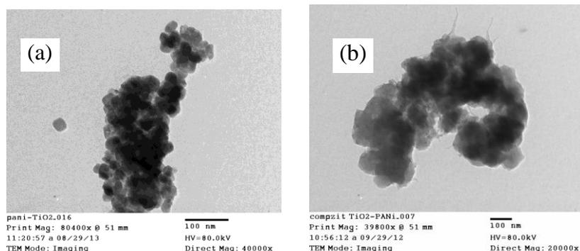
Fig. 1: TEM image of  $TiO_2$ -PANi composite (a) (A: ratio 1/6) and (b) (B: ratio 1/12)
