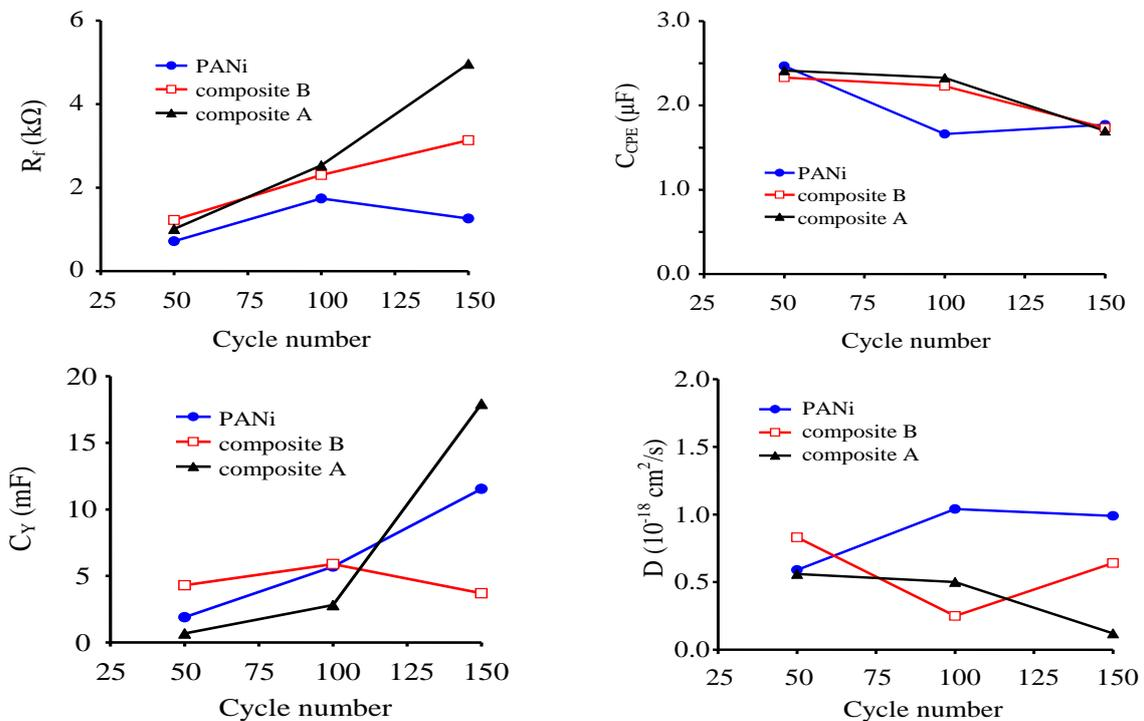
Figure 3: The dependence of some fitting electrochemical parameters on cyclic number applying in synthesis process of materials. The mass ratio of TiO<sub>2</sub> to aniline: 1/6 (composite A) and 1/12 (composite B)
