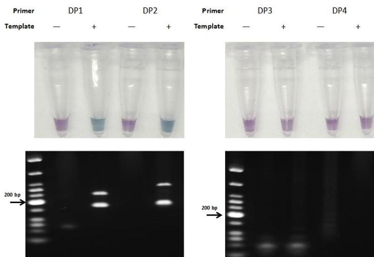
**Figure 2.** Primer set selection for multiplex RPA reactions. The reaction was incubated for 35 minutes at 39 °C. *V. parahaemolyticus* DNA sample extracted (10<sup>4</sup> copies/reaction) and WSSV synthetic target DNAs (10<sup>4</sup> copies/reaction) were used in the reaction. The reaction was incubated at 39 °C for 35 minutes. The results were analyzed using 0.08 mM EBT and 2.5% agarose gel electrophoresis. (+) and (-) represent the positive and negative samples, respectively.
