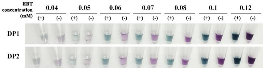
**Figure 3.** Optimization of EBT concentration. The reaction was incubated at 39 °C for 35 minutes. The indicated concentrations of EBT were used to analyze the reaction outcome. (+) and (-) represent the positive and negative control samples, respectively.
