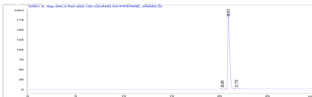
Figure 2. HPLC chromatogram of purified piperine showing approximately 96.7% of purity
