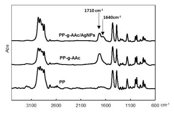
Figure 4. FTIR spectra of PP-g-AAc and PP-g-AAc/AgNPs samples.
