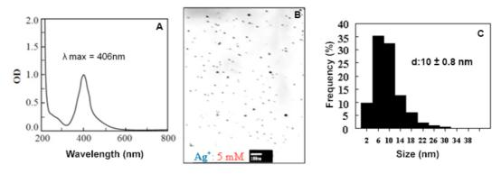
Figure 2. UV-vis spectrum (A), TEM image (B) and size distribution (c) of AgNPs prepared by γ-irradiation.
