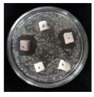
**Figure 7.** Inhibition zone test of untreated PP (a), PP-g-AAc (b), PP-g-AAc/AgNPs contained 132 ppm Ag (c) and 363 ppm Ag (e) and washed untreated PP immobilized with AgNPs (d).
