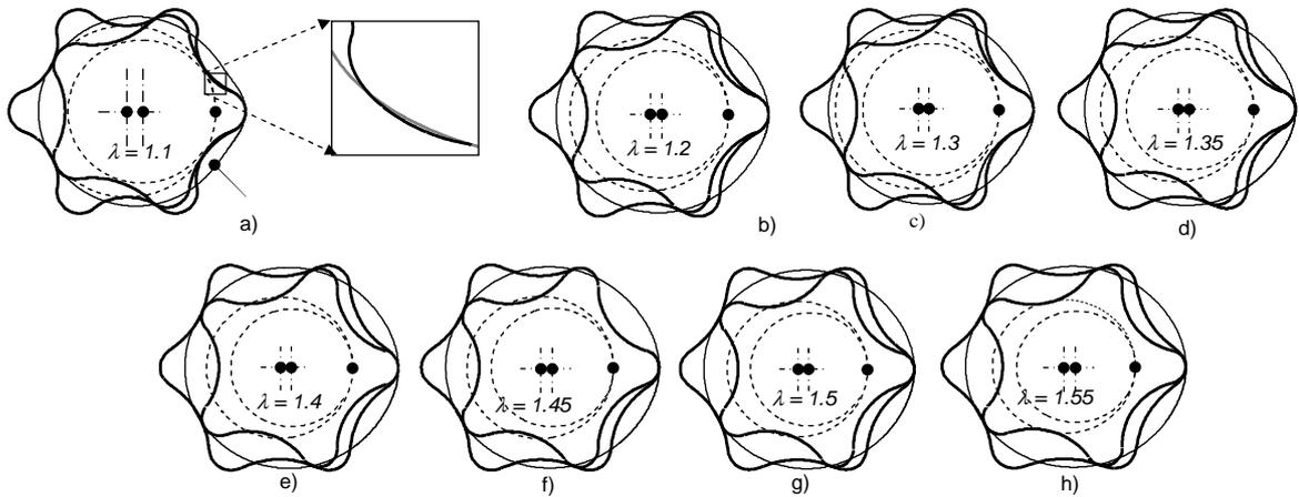
Figure 9. Gear-train with respect to  $\lambda$ .
