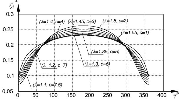
Figure 13. Sliding curve  $\xi_1$  with respect to  $\lambda$ ,  $c$ .
