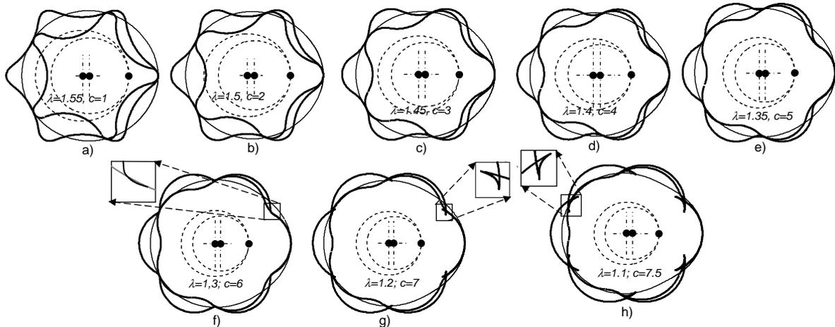
Figure 15. The gear pairs with respect to  $\lambda$  and  $c$ .
