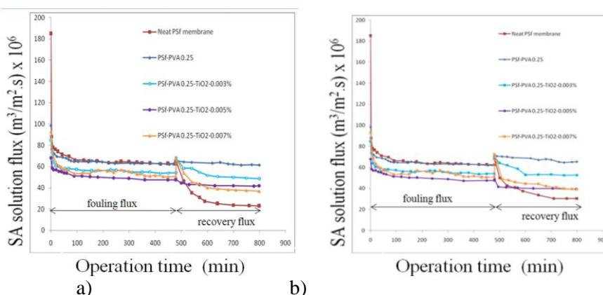
Figure 6. Flux for different membrane in sodium alginate filtration
