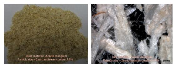
*Figure 2. A.mangium* sawdust with particle size < 2 mm; (left) optical camera; (right) optical microscope: Zeiss AXIO Imager.M2m.
