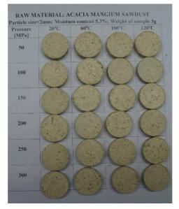
*Figure 4*. Tablets made from particle size < 2 mm.
