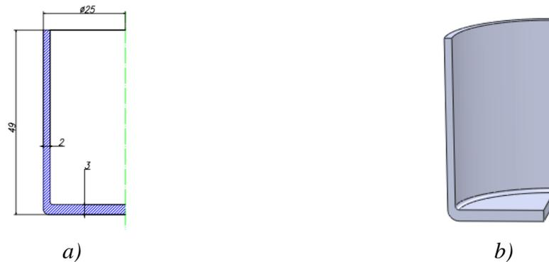
Figure 4. The axisymmetric detail: a) 2D drawing; b) 3D model.
