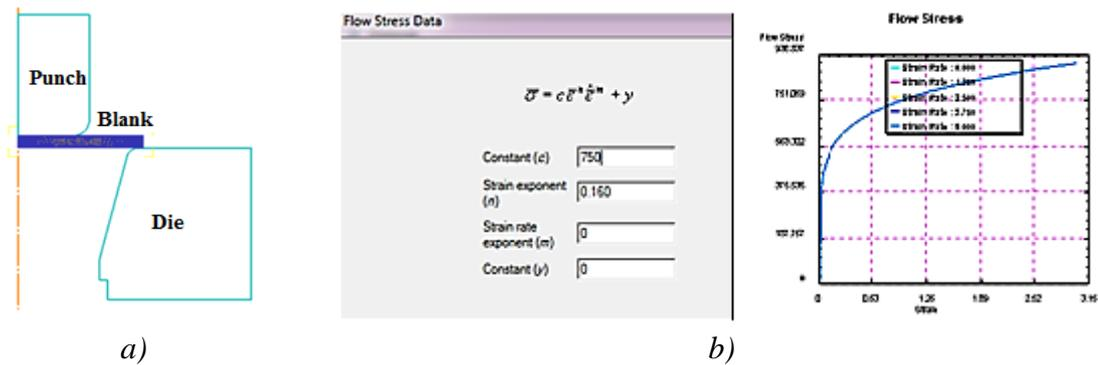
Figure 5. The geometry model (a), the material model (b).
