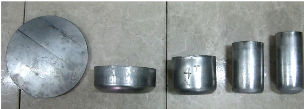
Figure 2. The combined drawing process [2].
