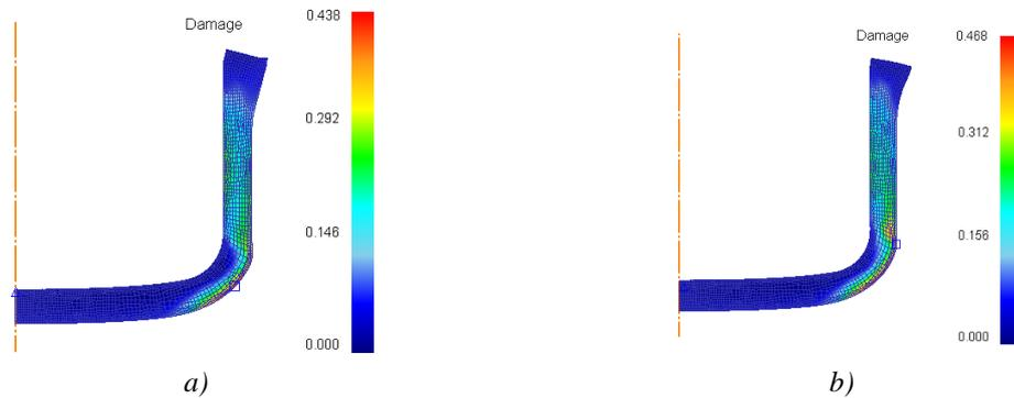
Figure 8 . The values of maximum strain effective when combined drawing with two types of die design parameters:
