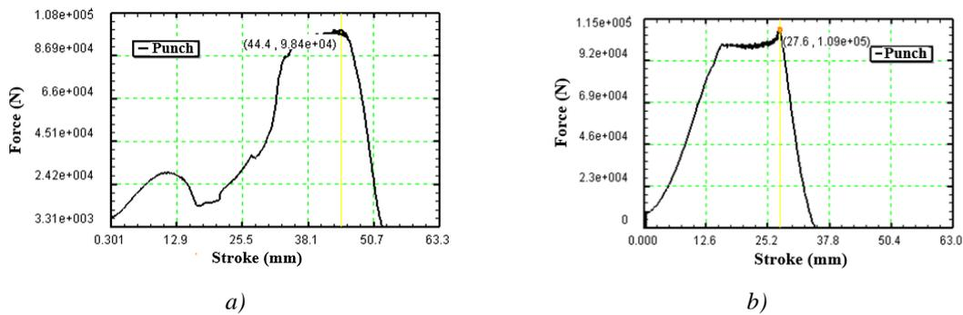
Figure 9. The drawing force is examine when combined drawing with two types of die design parameters: a) conical die; b) none conical die.
