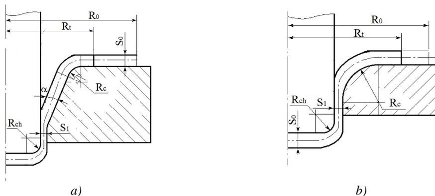
Figure 3. Two types of die design parameters. a) conical die; b) none conical die.
