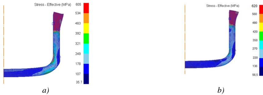
Figure 6 . The values of maximum stress effective when combined drawing with two types of die design parameters:
