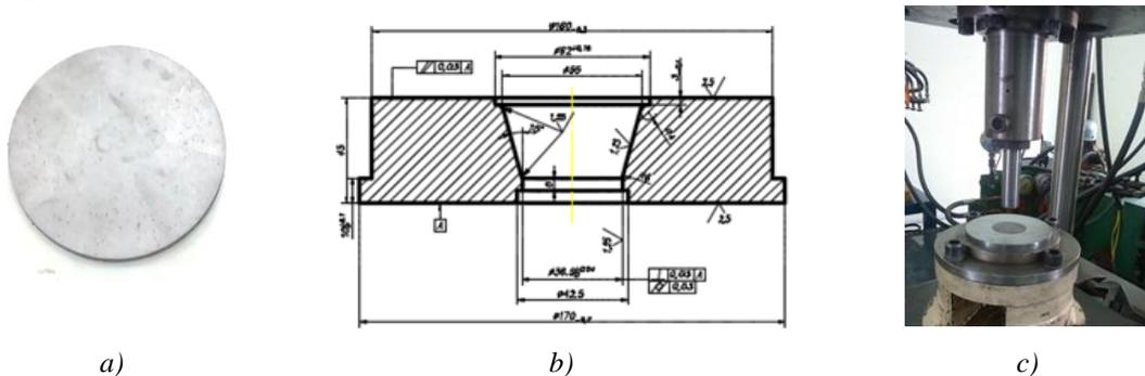
Figure 10. The blank (a), die (b), the tools when mounting on hydraulic presses YH32-100T (c).
