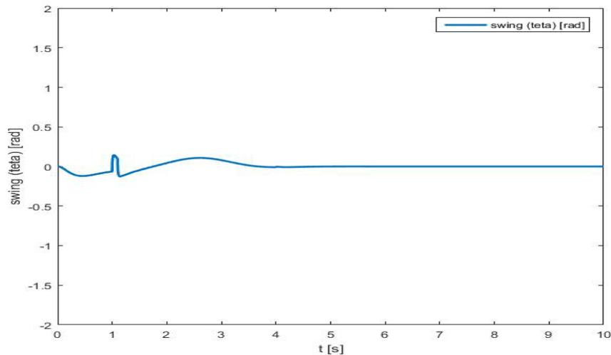
*Figure 9.* Swing angle of load when system is controlled by sliding mode controller combined with compensation anti-sway based on artificial neural network by PSO algorithm with the disturbance at time 1 [s].
