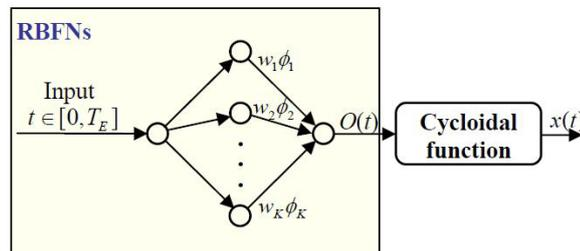
Figure 2. Radial Basis Function Neural Networks.
