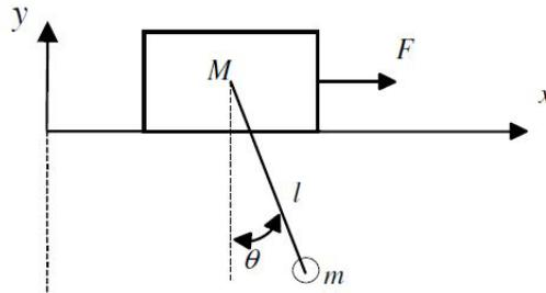
Figure 1. Overhead crane model.
