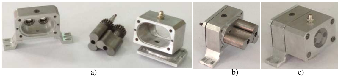
Figure 8. The prototype of the Roots pump.
