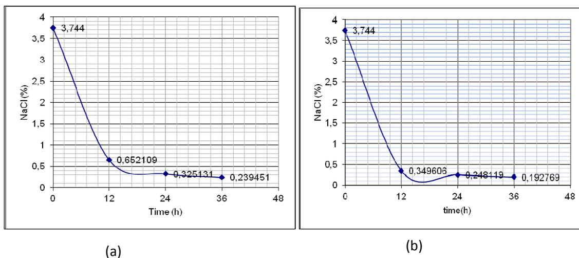
Figure 1. Salt removal by dialysis in static (a) and dynamic (b) conditions.
