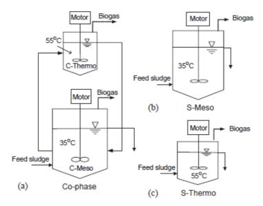
*Figure 6.* Anaerobic thermophilic pretreatment: (a) The temperature co-phase *AD* system; (b) The single-stage *MAD*; (c) The thermophilic AD processes [17].
