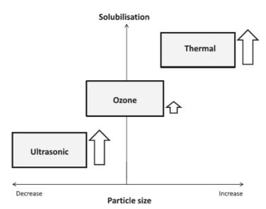
*Figure 12.* Qualitative pretreatment effects on *WAS* [4]. The arrows indicate the effect on biodegradability that was equally enhanced by *US* and thermal pretreatments and much less by ozonation.
