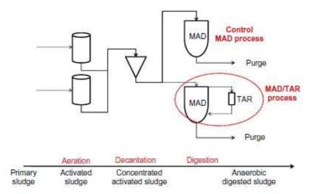
Figure 4. Aerobic hyper-thermophilic co-treatment [12].
