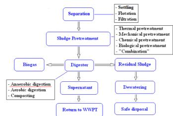
executive review and a short comparison of common sludge pretreatments, serving the selection of the most suitable technique for lab scale research and for subsequent actual application.
