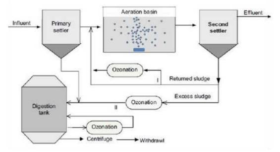
Figure 8. Application of ozonation for sludge disintegration [119].
