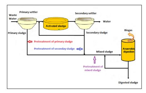
Figure 3. Sludge sources from classical wastewater treatment plants [4].
