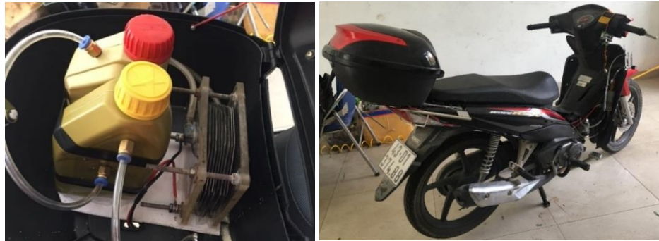
Figure 4. Installation of Dry-Type HHO Gas Generator into motorcycle.
