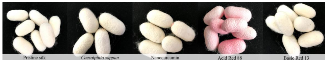
Figure 1. Self-dyed cocoons with various artificial (Acid Red 88, Basic Red 13) and natural ( Caesalpinia sappan , nanocurcumin) colorants.
