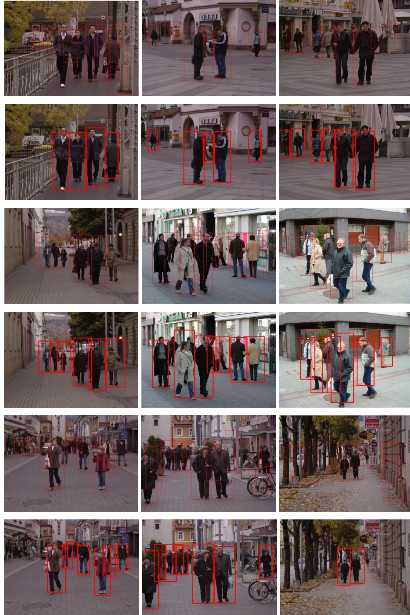
Figure 13. Result of pedestrian detection system test - HG stage (odd rows of images) and HV stage (even rows of images)
