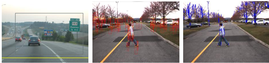
Figure 5. The region used to calculate average color of the road (left); Above and below regions used to calculate different average color (middle); Result of "colors difference method" (right)
