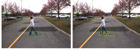
Figure 7. The ROI used for symmetry searching (left) and result of finding peaks (right)
