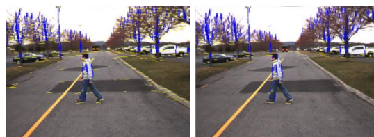
Figure 4. Result after repairing horizontal edges (left) and removing useless horizontal edges (right)
