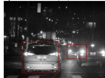
(d) False detection of light blobs of two vehicles at cross intersection as vehicle
