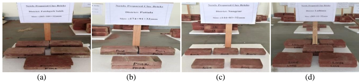
Figure 4. Newly prepared clay bricks (NPCB) from selected districts (thickness: 3 cm).
