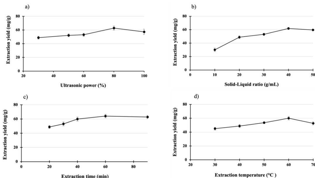
Figure 4. Effect of the single factor on the DO-R's extraction yield: a) Ultrasonic power, b) Solid-liquid ratio, c) Extraction time, and d) Extraction temperature.
