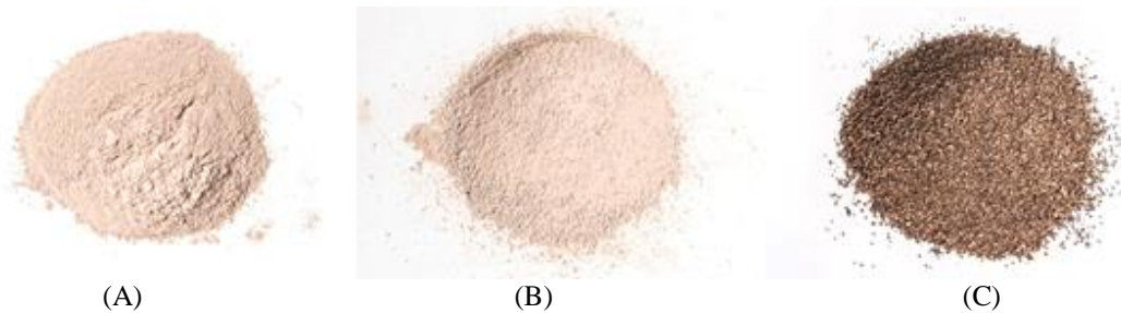
Figure 1. Commercial azomite rock of Azomite Mineral Products, Inc – USA (adapted from website [35]) : (A) Azomite Micronized D_{90} < 74 \mu\text{m} , (B) Azomite Field Grade 74\mu\text{m} < D_{90} < 3 \text{ mm} , (C) Azomite Granulated D_{90} > 3 \text{ mm} .
