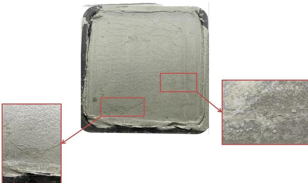
Figure 13. Visual inspection of coated sample of mortar slab with acrylic-styrene film
