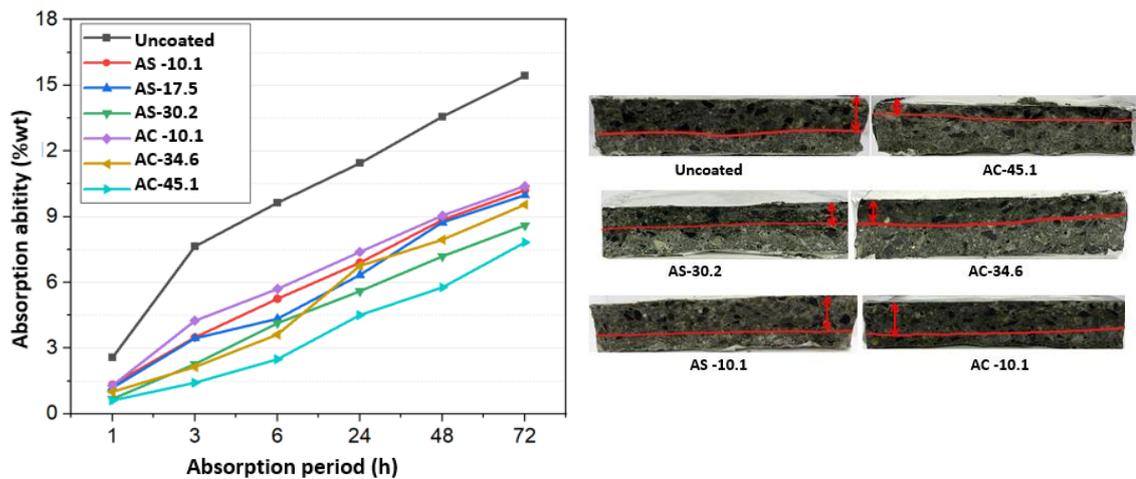
Figure 9. Water absorption of mortar sample due to capillary (note: AS = acrylic styrene; AC = acrylic).
