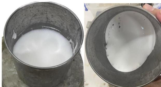
Figure 3. Milky white solution of acrylic-based emulsion with different solid contents.
