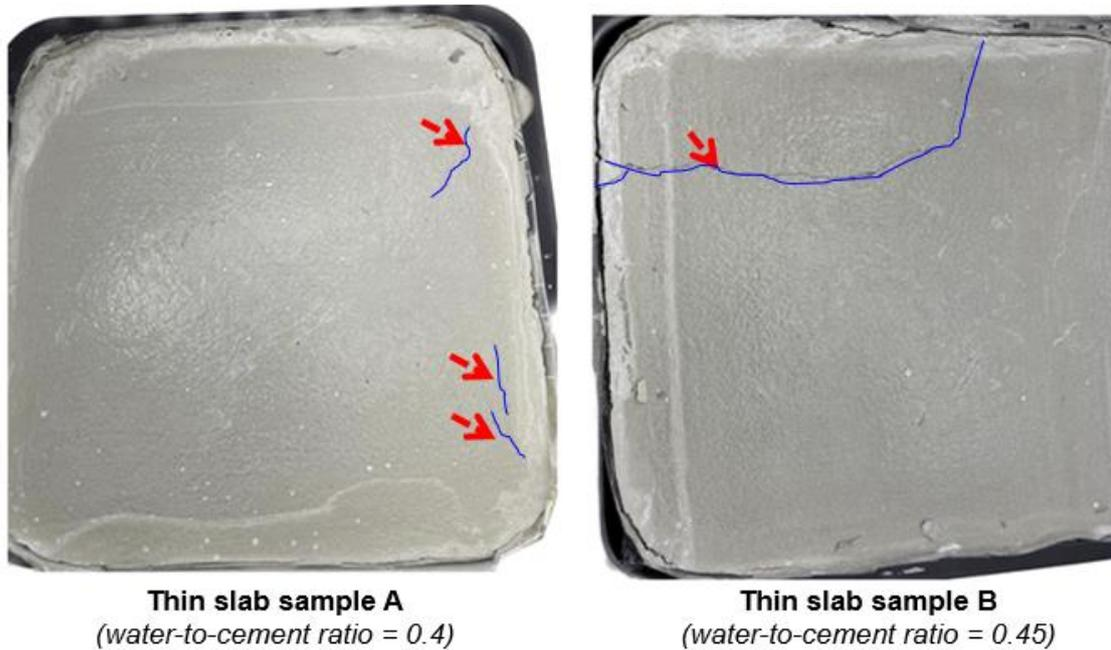
Figure 11. Two series of thin slab sample A and B with different water-to-cement ratios and generated cracks (blue) after 24 hours of curing period with sprayed water for moisturing
