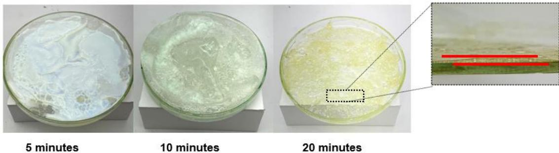
Figure 6. Acrylic emulsion after drying 5, 10 and 20 minutes at 120 °C in a petri dish.
