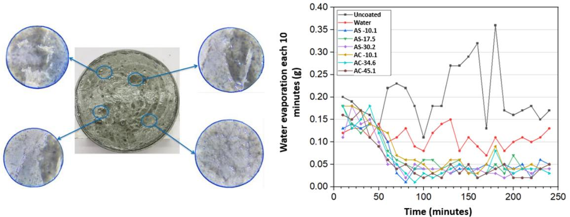
Figure 7. (left) Visualisation of coating film on the surface of cement paste; (right) Water evaporation rate each 10-minutes interval during the drying process (note: AS = acrylic styrene; AC = acrylic).
