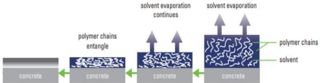
Figure 2. From left to right: Illustration of solvent evaporation and film-forming process of acrylic-based emulsion on the concrete substrate [6].
