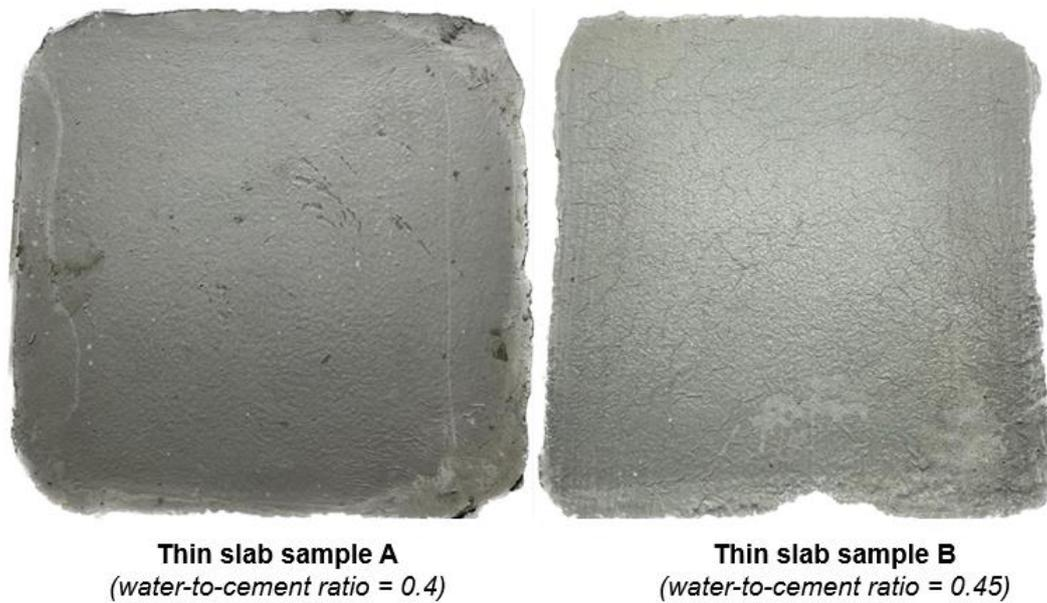
Figure 12. Two series of thin slab sample A and B with different water-to-cement ratios after 24 hours of curing period with sprayed acrylic-styrene emulsion (AS) 17,5 %wt of solid content
