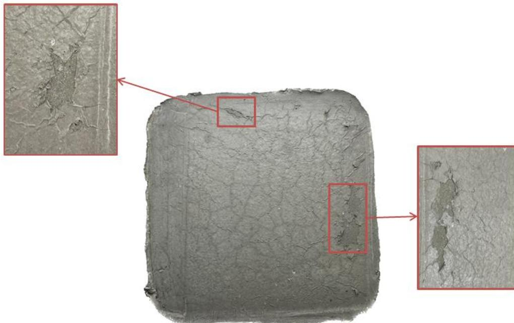
Figure 15. Visual inspection of coated sample of mortar slab with acrylic film
