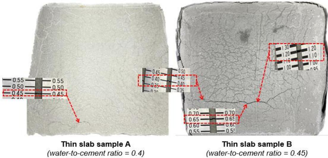
Figure 10. Two series of thin slab sample A and B with different water-to-cement ratios and generated cracks due to shrinkage during 24 hours of curing period
