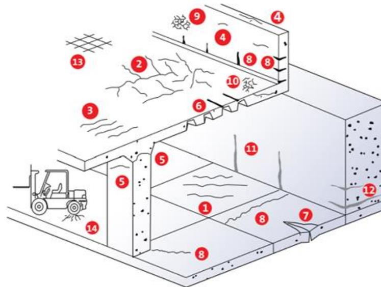
*Figure 1.* Common types of cracks in cement-concrete structures and their causes. (Plastic settlement: 4, 5, 6, 13; Plastic shrinkage: 1, 2, 3; Early thermal contraction: 11, 12; Long-term drying shrinkage: 8; Cracking: 9, 10; Cracks due to overloading: 14) [2].
