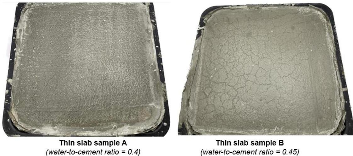
Figure 14. Two series of thin slab sample A and B with different water-to-cement ratios after 24 hours of curing period with sprayed acrylic emulsion (AC) 34.6 % wt of solid content
