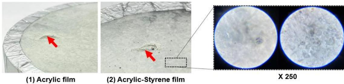
Figure 8. Formed film layer on the cement mortar substrate due to sprayed emulsion of acrylic
