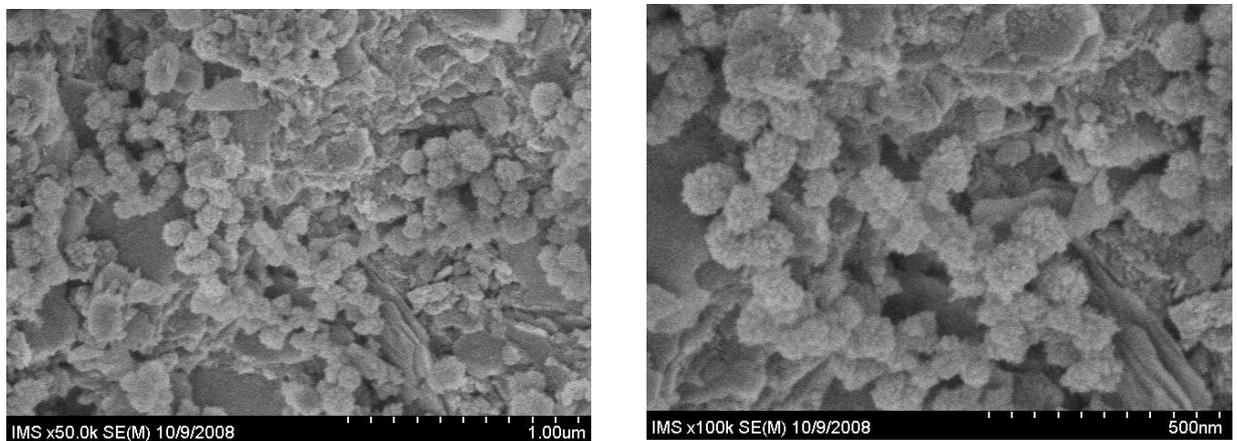
*Figure 4. SEM image of denaturated laterite surface after nano MnO<sub>2</sub> coating*
