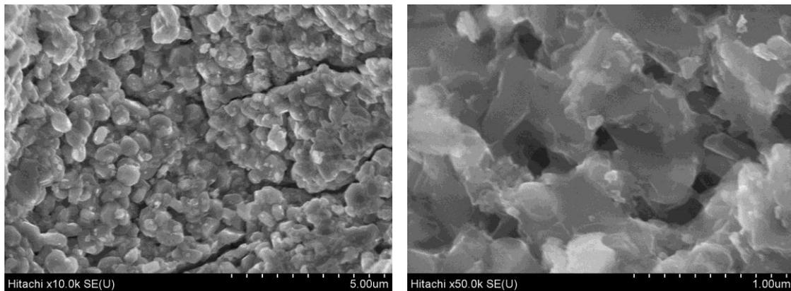
*Figure 4. SEM image of denaturated laterite surface before nano MnO<sub>2</sub> coating*
