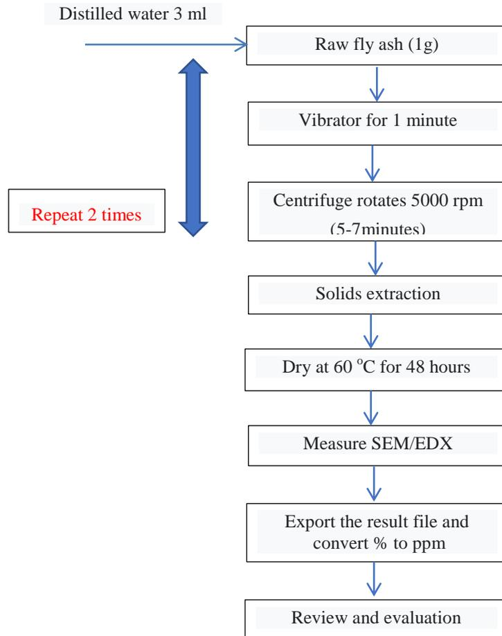
Figure 3. Process of analyzing fly ash composition by SEM/EDX method.
