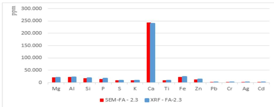
Figure 4. Comparison chart of fly ash composition of Soc Son Waste Power Plant - phase 2 by SEM/EDX and XRF.
