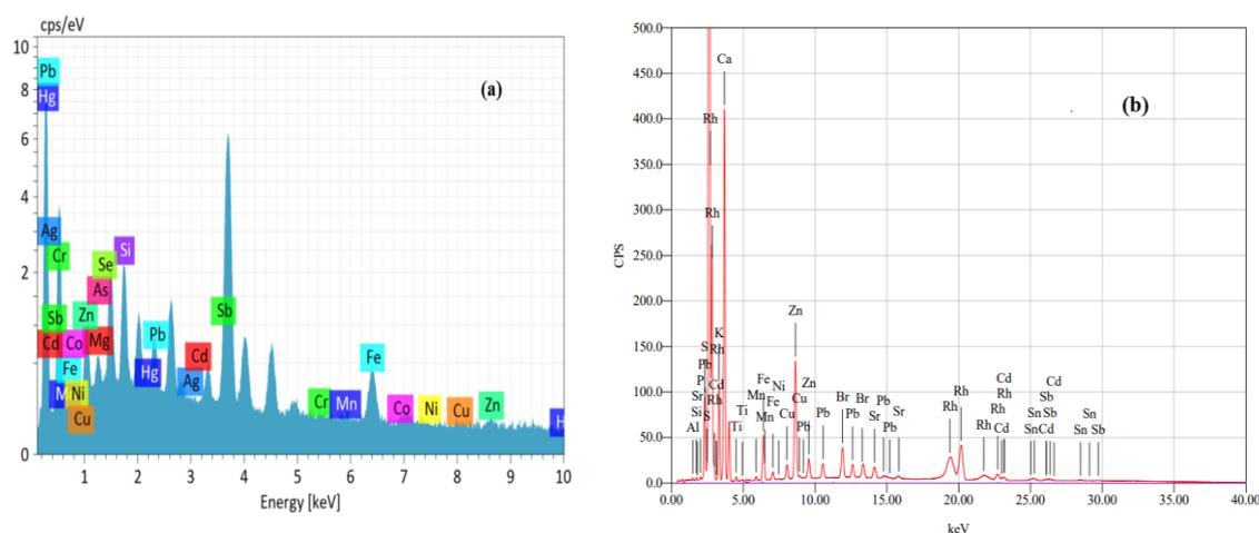
Figure 2. The Energy dispersive X-ray spectrum of the fly ash by SEM/EDX (a) and XRF (b).
