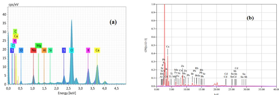
Figure 5. The energy dispersive X-ray spectrum of the fly ash by SEM/EDX (a) and XRF (b).
