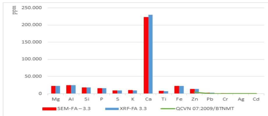
Figure 6. Comparison chart of fly ash composition of Soc Son Waste Power Plant - phase 3.
