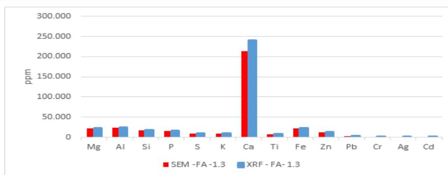
Figure 1. Comparison chart of fly ash composition of Soc Son Waste Power Plant - phase 1 by SEM/EDX and XRF.
