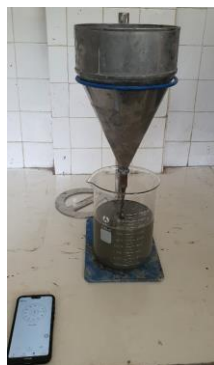
Figure 4. A photo of Marsh cone to measure the flowability of UPPCP (left) and an example of the determination of SP saturation point using Marsh cone for w/b ratio of 0.20 and 30% BFS (right).
