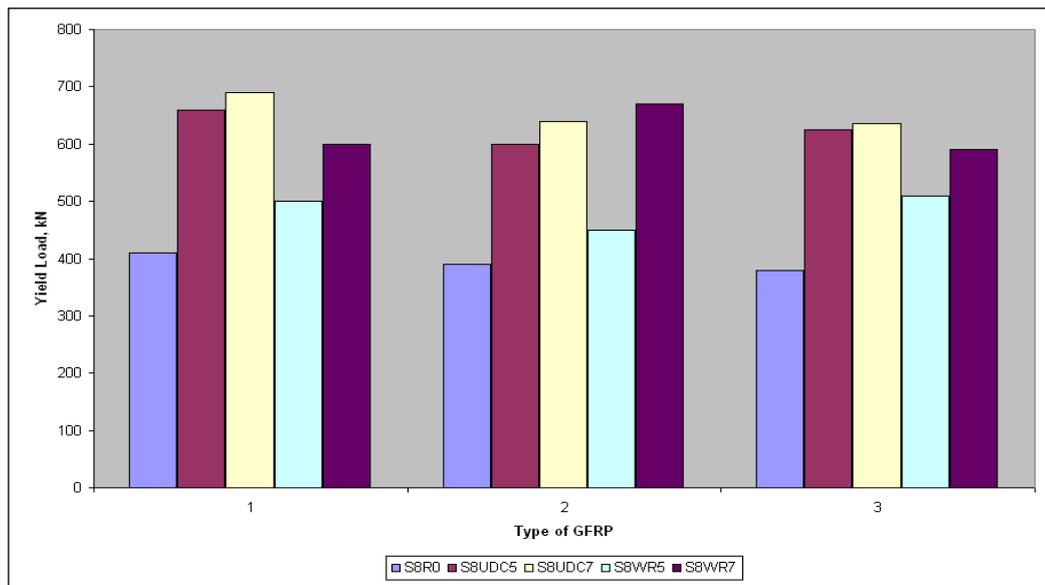
Figure 6. Yield load with different types of GFRP and thickness.
