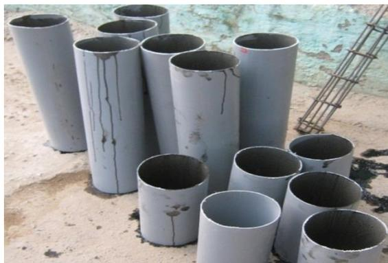
Figure 1. PVC pipes cut-to-size for casting.
