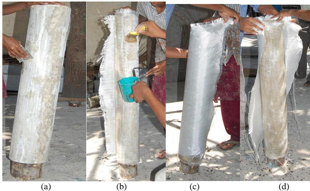
*Figure 3.* GFRP wrapped specimens: (a) After grinding, (b) Receiving layer of GFRP with epoxy resin, (c) Cured specimens, and (d) Receiving another layer of GFRP
