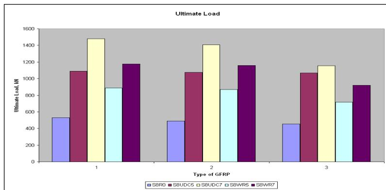
Figure 7. Ultimate load with different types of GFRP and thickness.
