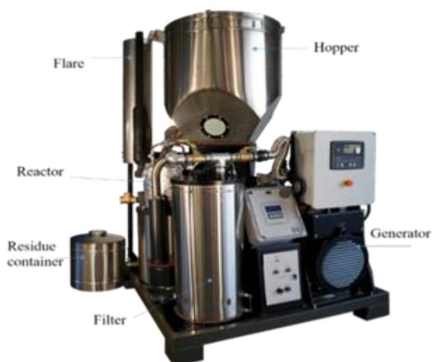
Figure 2. The commercial PP20 gasifier
