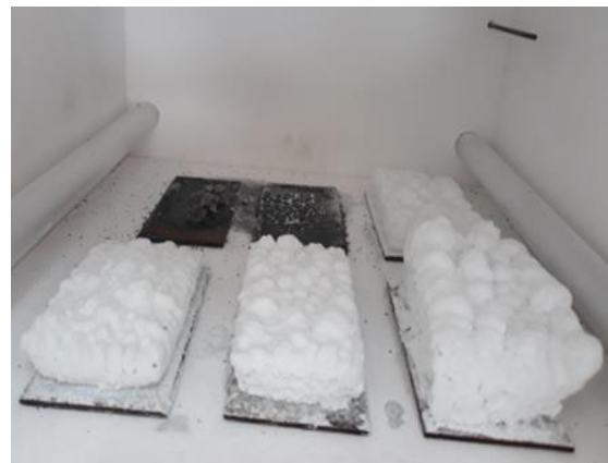
Figure 2. Coating samples after combustion.
