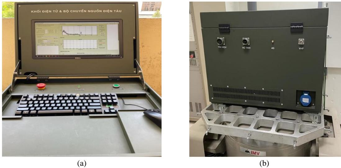
Figure 5. The electronic and power adapter block after fabrication and integration: (a) in actual measuring and (b) in vibration testing.
