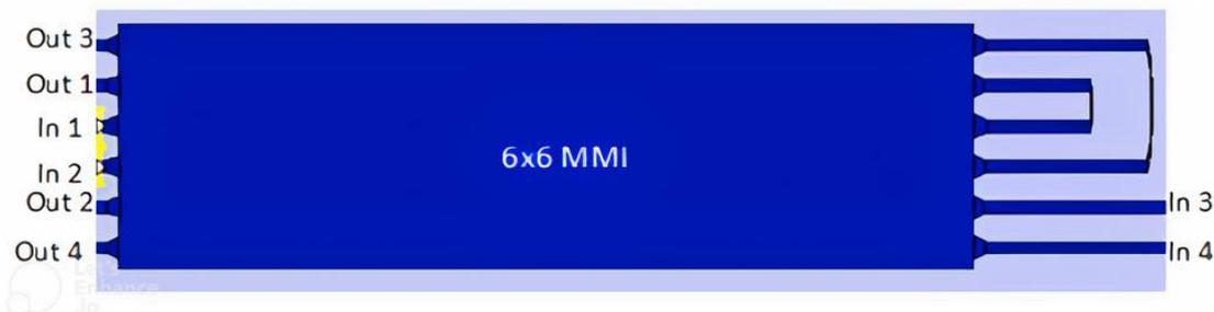
Figure 3. Photonic circuit for implementing the 4-point Haar transform using 6x6 MMI coupler.
