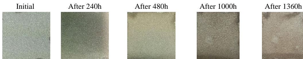
Figure 7. Surface change of Al-Mg coating sample during the salt spray test.
