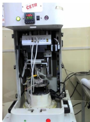
Figure 8. Evaluating properties of lubricating film layer based on the pin-on-flat model.
