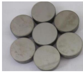
Figure 3. Specimens with CrN coating on SKD11 steel.
