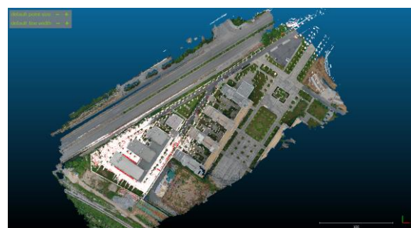
Figure 5. Matching demonstration between point cloud map of laser scanning and photogrammetry.
