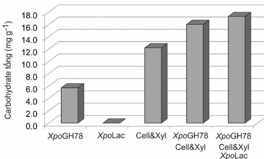
*Figure 2.* Sum of the released carbohydrates from milled rape straw after treatment with different enzymes (*XpoGH78*, *XpoLac*, and Cell&Xyl) as single applications, and in two enzyme combinations [(i) *XpoGH78* and Cell&Xyl; (ii) *XpoGH78*, Cell&Xyl, and *XpoLac*]. The values are corrected by the sugar amounts in the corresponding controls containing heat-denaturated enzymes.
