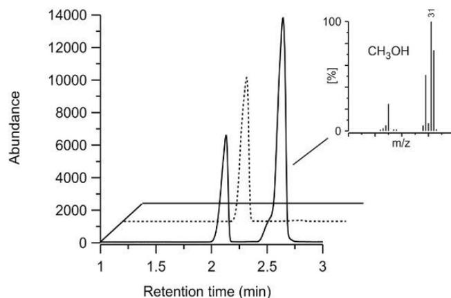
Figure 3. GC-MS elution profile of the enzymatic demethylation of rape straw (solid line) after 48 hrs of incubation. Control without enzyme (dashed line) insert shows the mass spectrum of biomethanol as the reaction product.
